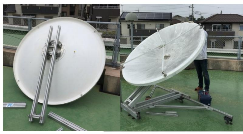
Reference Antenna is prepared by recycling use of 1.6m dish used for former GALA-V
