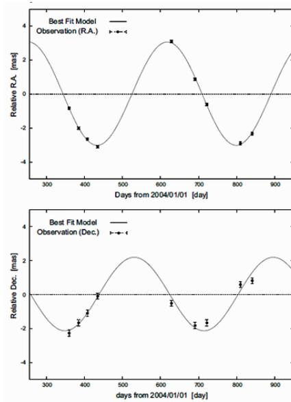
VERA monitors the separation angle between two radio-stars, MASER-emitting molecule cloud and Quasar, for more than two years, and determines a distance to the MASER emitting sources by annual parallax.
